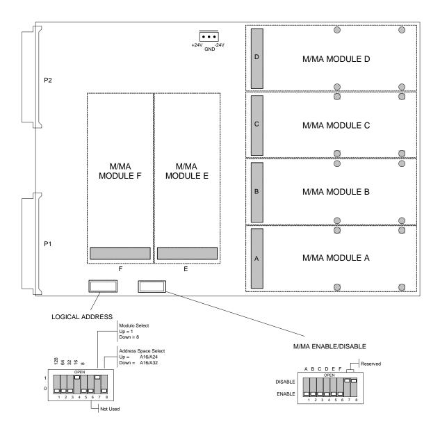
Figure 4. Hardware Configurable Controls
