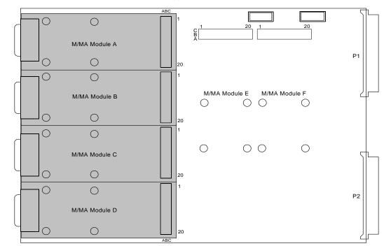
CONFIGURATION FOR FOUR (4) M/MA MODULES WITH FRONT PANEL ACCESS
