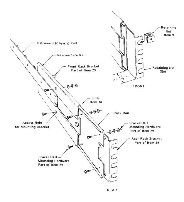
Figure 2-4, Slide and Bracket Components(9U Rack Mount Mainframe)
