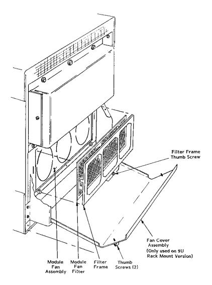
Figure 7-2, Cleaning The Module Fan Filter
