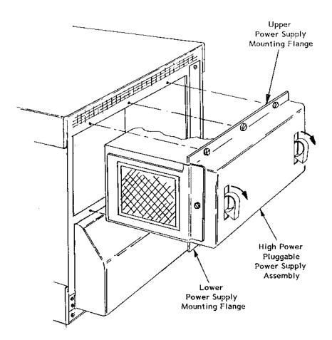
Figure 7-6, Removing The Power Supply
