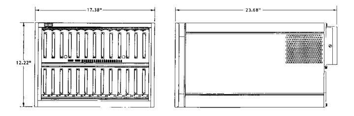
Figure A-2, Front View and Side View of Bench Top (7U) 1261B Mainframe
