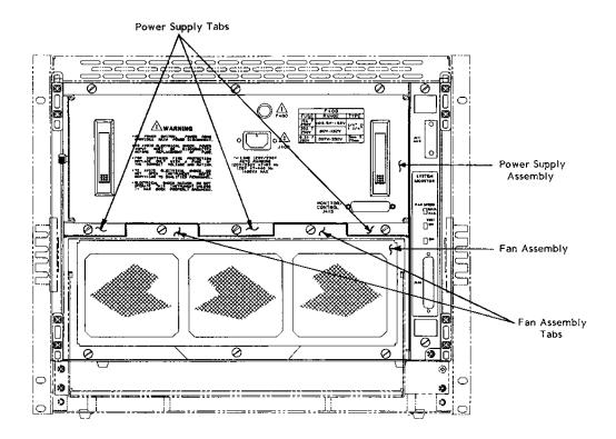
Figure 7-4, Aligning The Module Fan Assembly
