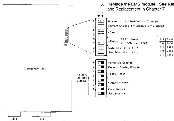
Figure 2-12, Setting the Enhanced Monitoring System Configuration Switch
