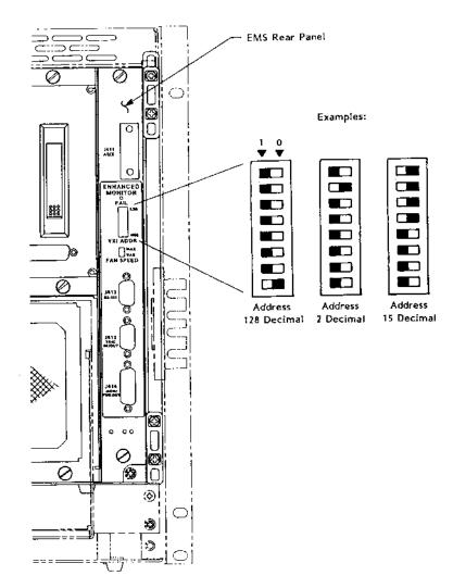
Figure 2-11, Setting The Enhanced Monitor VXI Logical Address
