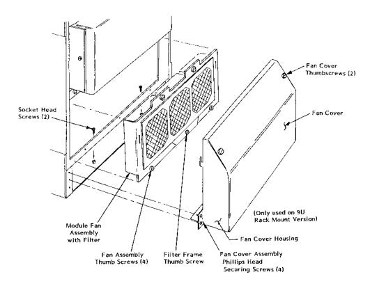
Figure 7-3, Module Fan Assembly Detail
