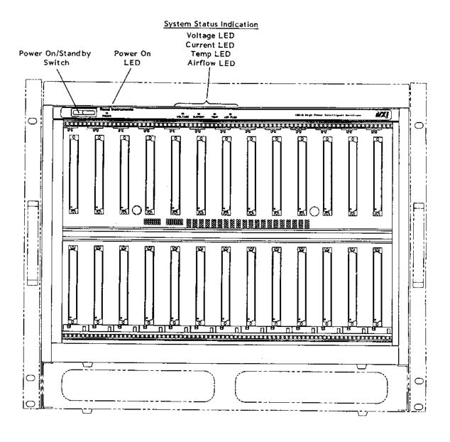
Figure 3-1, 1261B Front View With Standard Monitor
