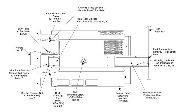
Figure 2-5, Preparing The Mainframe For Rack Mounting
