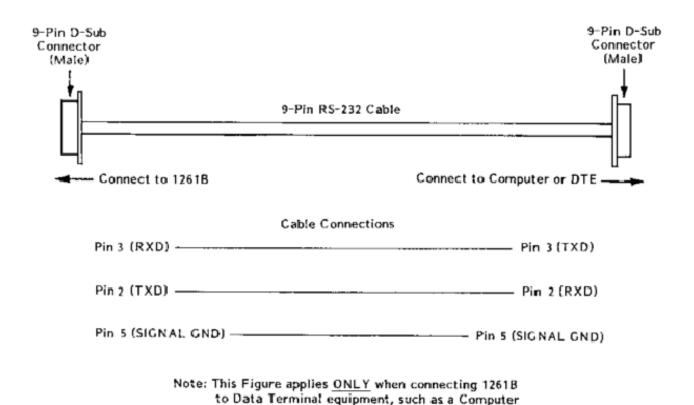
Figure 2-14, RS-232 Connections With a Computer, Data Terminal or Modem
