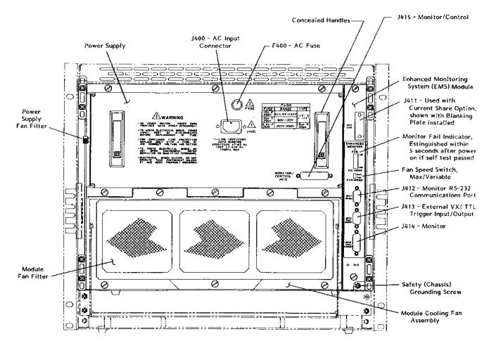
Figure 3-4, Rear View With Enhanced Monitor
