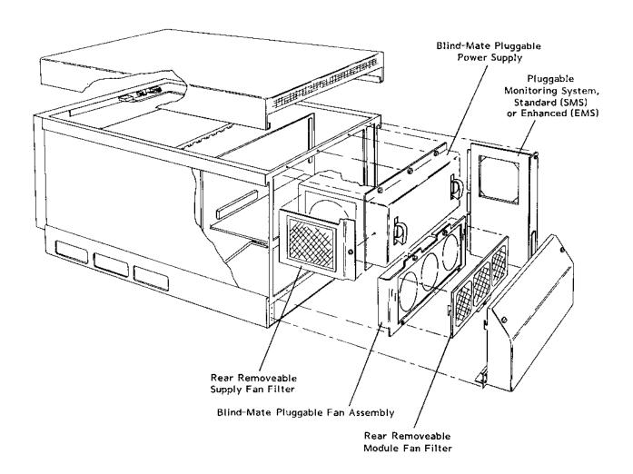
Figure 1-3, Modular Service Friendly Mainframe Design Features
