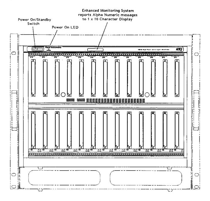
Figure 3-3, Front View With Enhanced Monitor
