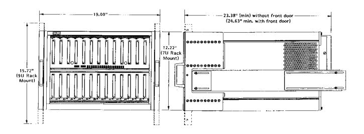
Figure A-3, Front View and Side View of 1261B Bench Top Model With 7U and 9U Rack Mount Ears
