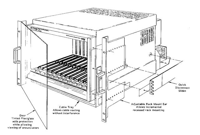
Figure 1-8, Rack Mount and Cable Tray Option Components
