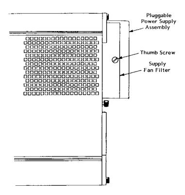
Figure 7-1, Cleaning The Supply Fan Filter
