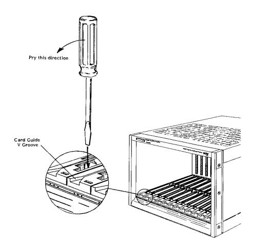
Figure 7-10, Card Guide Removal and Replacement
