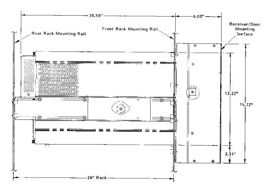
Figure A-5, Side View of 1261B 7U Mainframe With Option 54-1 Installed
