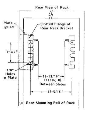
Figure 2-6, Rear End Slide Mount Rack Dimension
