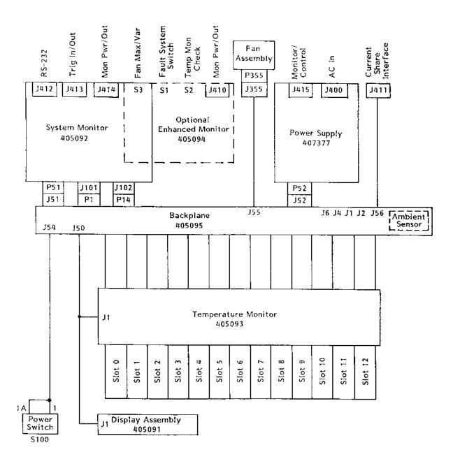
Figure 6-1, Functional Block Diagram For 1261B Chassis
