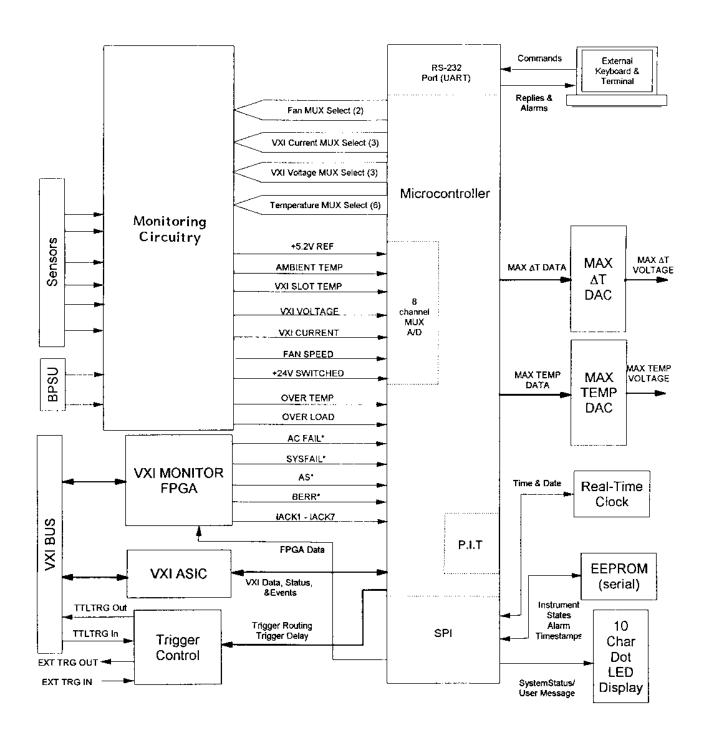
Figure 6-2, Enhanced Monitoring System Module Block Diagram
