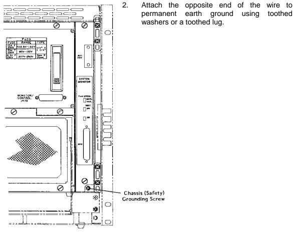
Figure 2-9, Connecting Safety Ground
