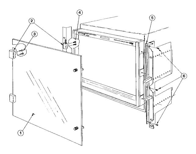
Figure 2-8, Installing Rack Door
