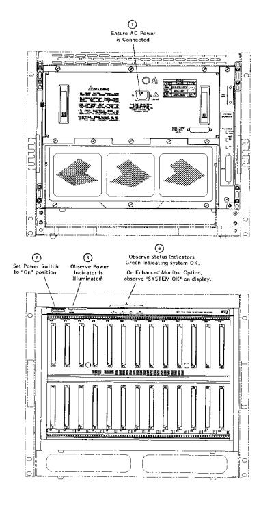
Figure 3-5, Powering On The Mainframe
