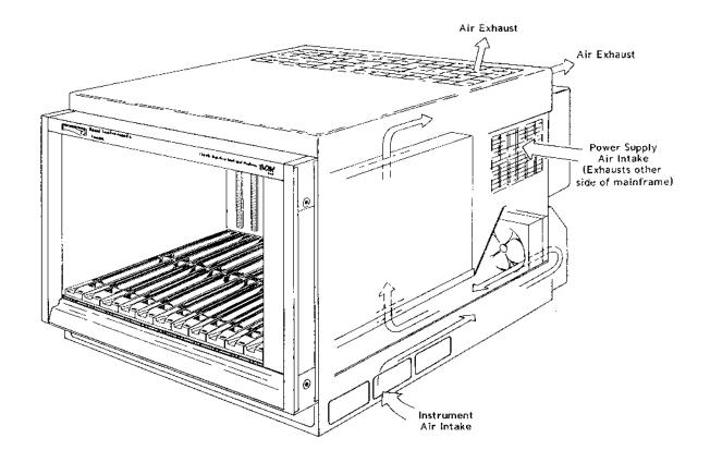
Figure 1-6, 1261B Rack Mount Mainframe Positive Pressure Cooling System
