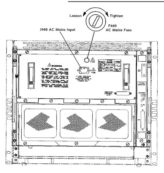
Figure 7-9, Removing and Replacing The AC Mains Fuse
