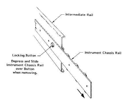
Figure 2-7, Instrument Rail Removal
