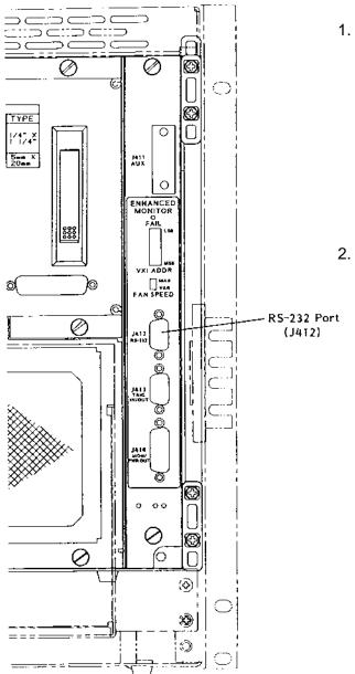
If factory default RS-232 setting is incompatible with your computer, (data terminal, or modem), perform the procedure described in Figure 2-12 Setting Enhanced Monitoring System RS-232 Configuration Switch.
