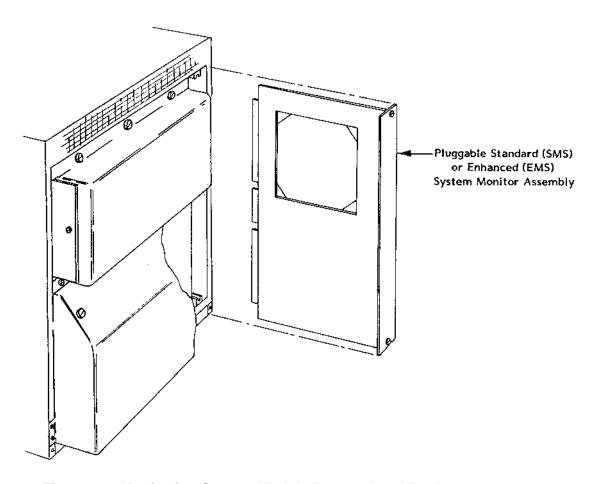
Figure 7-8, Monitoring System Module Removal and Replacement
