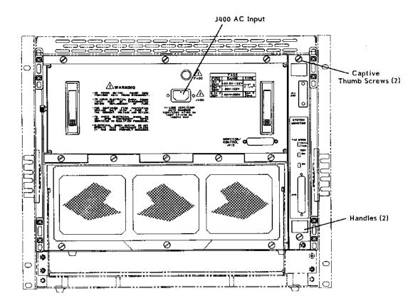
Figure 7-7, Monitor System Module Rear View
