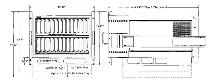
Figure A-4, Front View and Side View of 1261B Rack Mount Model With Rack Mount and Cable Tray Options
