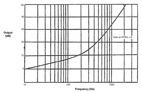
Figure 3-4, Filter 3 Equalizer Frequency Response
