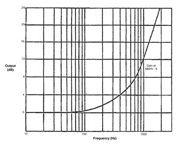
Figure 3-2, Filter 1 Equalizer Frequency Response
