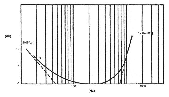
Figure 3-3, Filter 2 Equalizer Frequency Response
