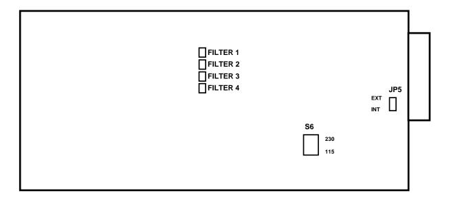
Figure 3-1, 200B Printed Circuit Board Layout
