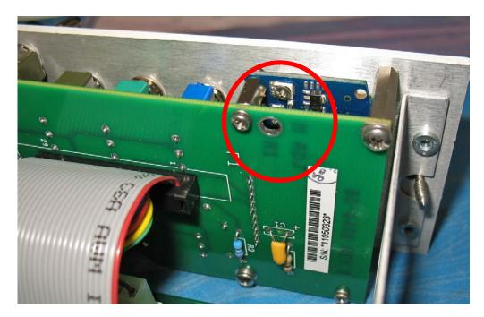
Figure 4-2, DVM Adjustment Resistor R1
