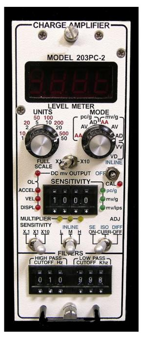
Figure 1-1, 203PC-2 Charge Amplifier
