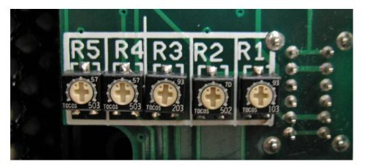
Figure 4-1, Potentiometer Adjustment Locations
