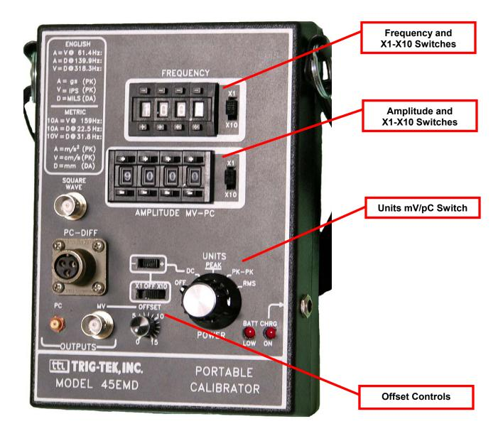
Figure 2-1, 45EMD Control Switches
