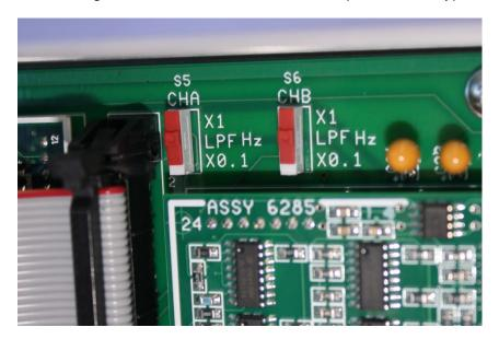
Figure 2-2, Low-Pass Cutoff X1-X0.01 Switch
