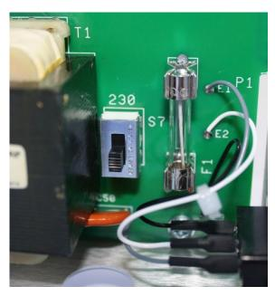
Figure 2-1, Dual Power Mode Switch (shown set to 115 V)
