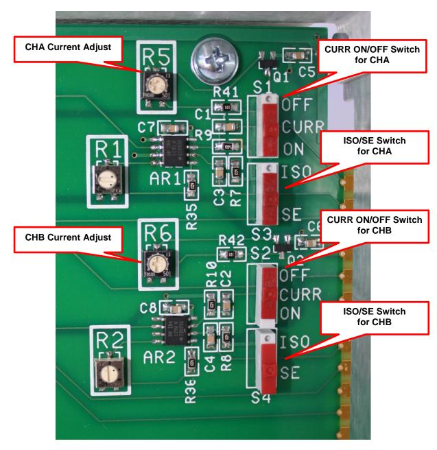
Figure 2-3, SE-ISO and CURR ON/OFF Switches
