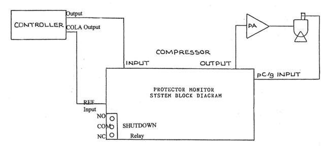
Figure 2-1, Simplified System Block Diagram
