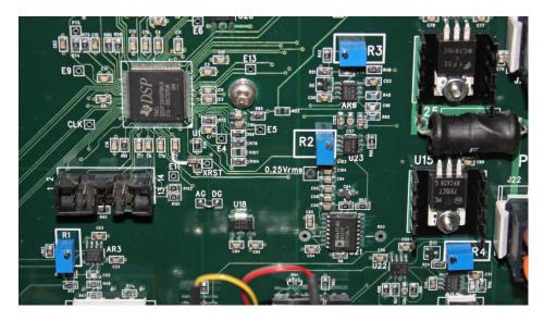
Figure 4-1, Main Board Variable Resistor Locations
