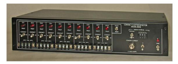
Figure 1-2. Trig-Tek 850B Contact Chatter Detector
