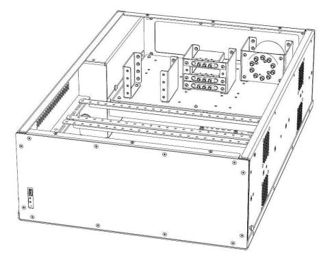
Figure 2-16, Installed Accessory Plate and Components (Example)
