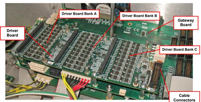
4. Connect power cable from the power supply to the driver board.
