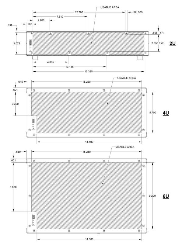
Figure 2-1, External Panel Usable Mounting Area – Front Views
