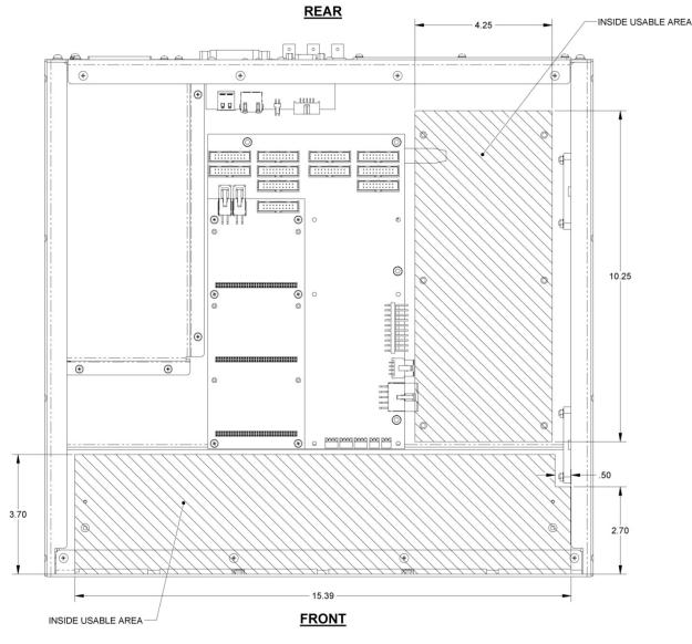
Figure 2-3, Internal Usable Mounting Area – 2U
