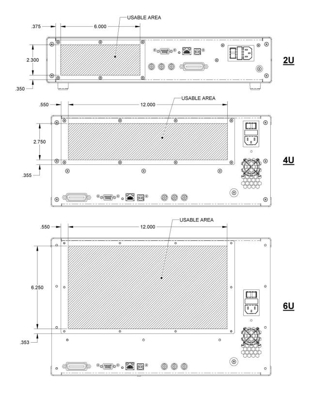
Figure 2-2, External Panel Usable Mounting Area – Rear Views
