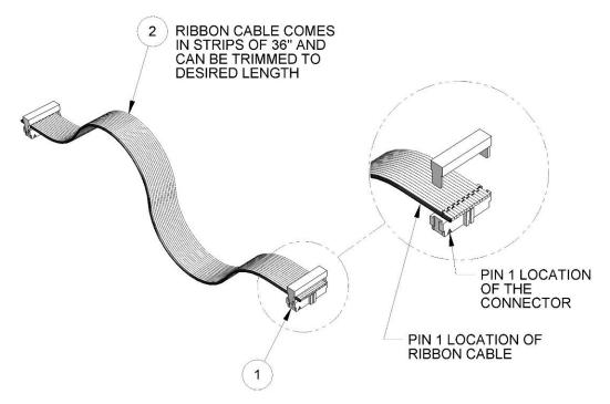
Figure 2-19, Attaching the Ribbon Cable Connector
