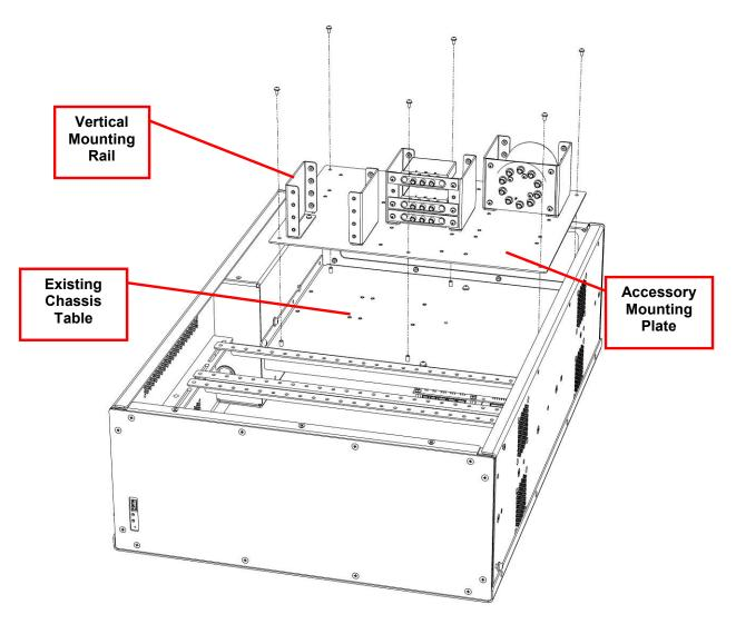
Figure 2-15, Inserting Accessory Plate and Mounting Rails
