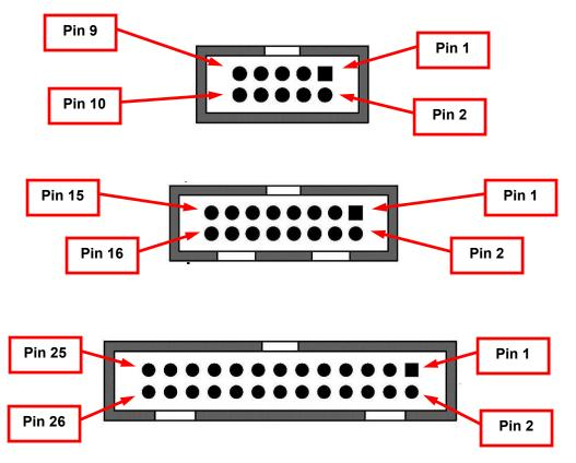
Figure C-9, Adapter Board Connectors and Pin Numbering
