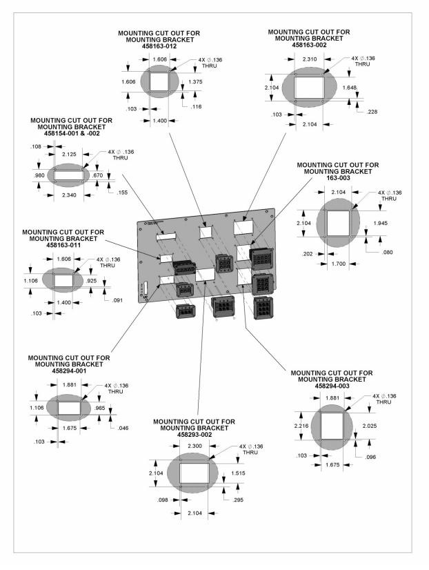
Figure B-3, Exterior Mounting Bracket Cut Out Specifications
