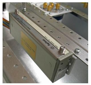
Figure 2-14, Examples of Installing Components on Rails
