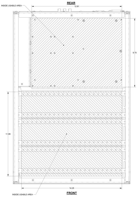
Figure 2-4, Internal Usable Mounting Area (Top View) – 4U and 6U
