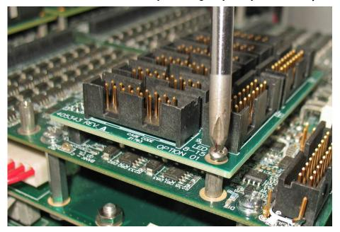
Figure 2-10, Adapter Board Location on Driver Board
