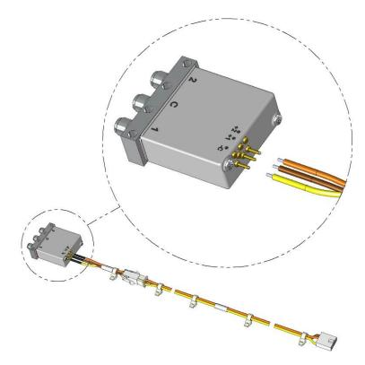
Figure 2-18, Attaching Pigtail Connectors
