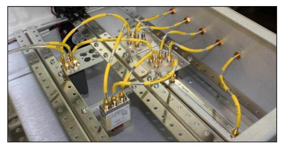
Figure 2-22, 1257A with Components Cabled to a Customized Front Panel (Example)
