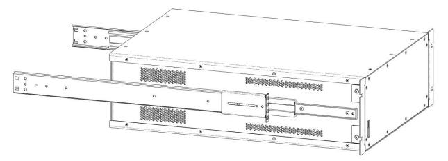
Figure F-2, Rack-Mounting Slides Attached to 1257A (Appearance Typical)
