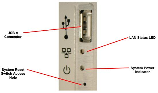
Figure 1-5, 1257A-D Front View Detail
