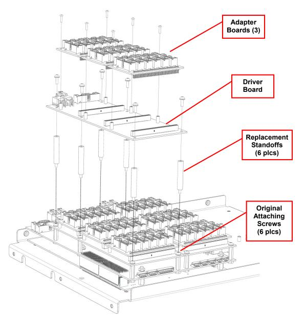
Figure 2-9, Driver Board Stacking
