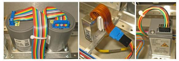
Figure 2-17, Connecting Cables to Components (Examples)
