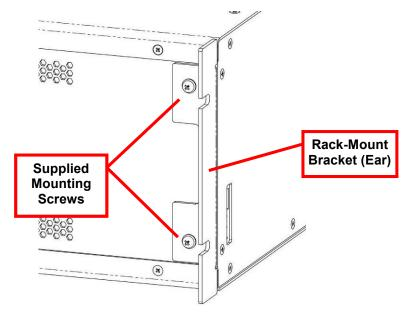
Figure F-1, Attaching Rack Mount Brackets (Appearance Typical)
