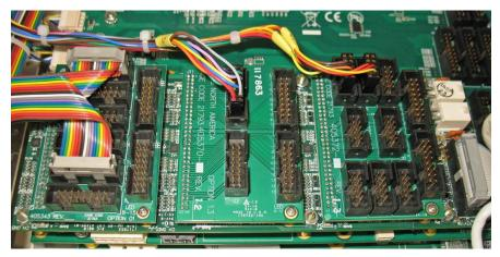
Figure 2-20, Cabling Components to Adapter Boards (Examples)
