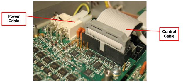
Figure 2-8, Power and Control Cables
