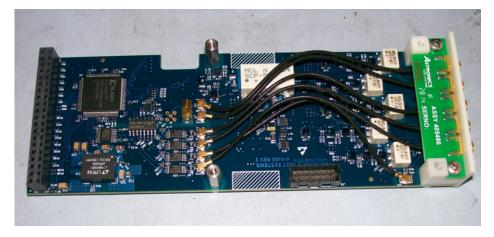
Figure 5-2, M1712 PWA, Component Side
