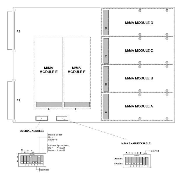
Figure 2-4, VX405C Hardware Configurable Controls
