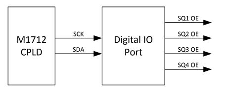
Figure 5-6, Square Wave Output Enable Control
