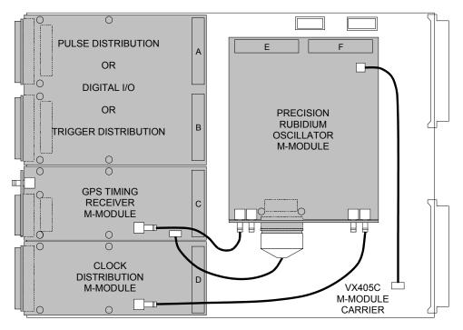
Figure 2-1, 3352A M/MA Configuration Diagram
