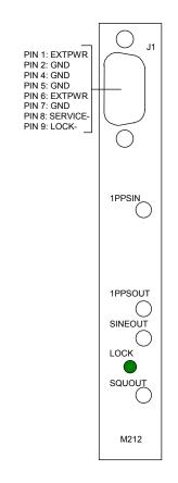
Figure B-1, M212 Front Panel I/O Signals
