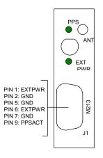
Figure C-1, M213 Front Panel I/O Signals
