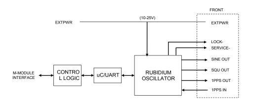
Figure 3-2, M212 Functional Block Diagram
