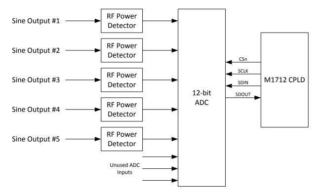
Figure 5-5, Sine Wave RF Power Monitors
