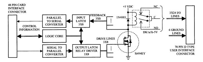
Figure 2-2, 1260-116 Block Diagram
