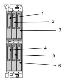
Front View – Module Addresses for 1260-100 Carrier
