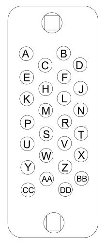
Figure 2-3, Front-Panel Connector Pin Numbering
