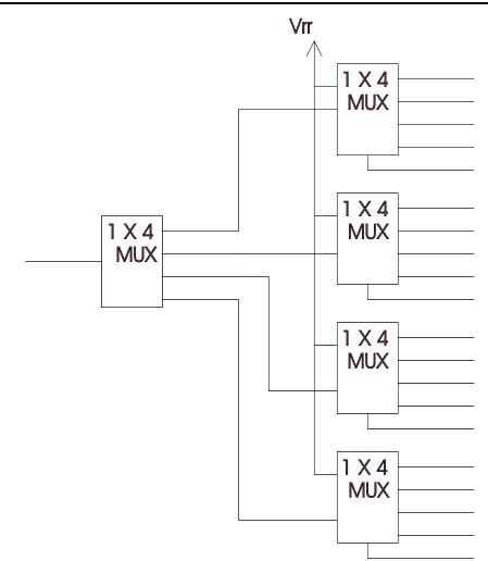
Figure 2-2, Typical Cascade Configuration
