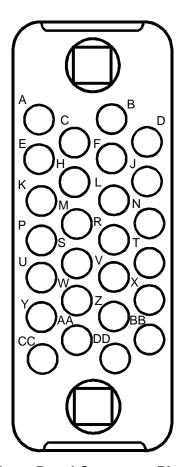
Figure 2-1, Front-Panel Connector Pin Numbering
