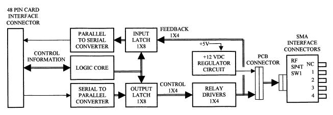
Figure 2-3, 1260-164AH Block Diagram
