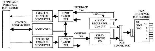
Figure 2-6, 1260-164BH Block Diagram
