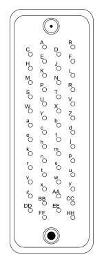
Figure 2-3, Front Panel Connector Pin Numbering
