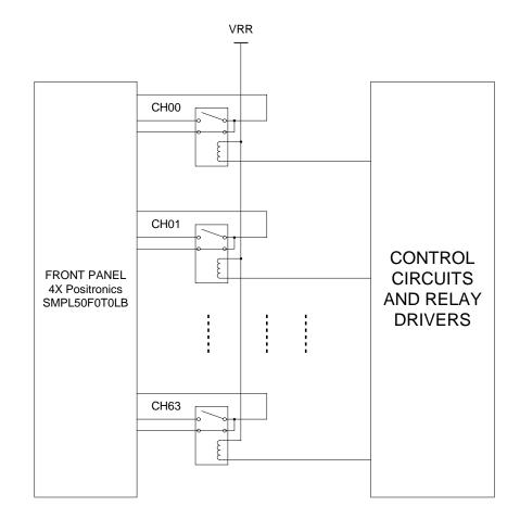
Figure 2-1, 1260-16A, Switch Block Diagram
