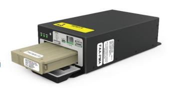
The CabinEdge-2 product is a Solid State Drive Content Loader (SSDCL) with a SATA Based Removable SSD Module with up to 7.6TB SSD storage. The product loads digitally stored, encrypted content in the background in an unattended fashion.
