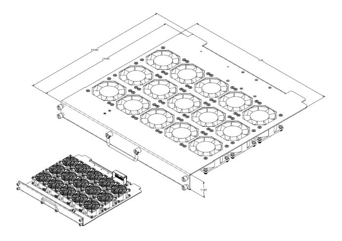
Figure 5-1, Module Fan Assembly Detail
