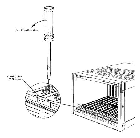
Figure 5-3, Card Guide Removal and Replacement
