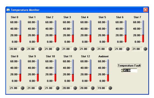
Figure 6-5, Per Slot Temperature Monitoring
