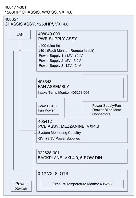
Figure 4-1, 1263HPf Chassis Functional Block Diagram
