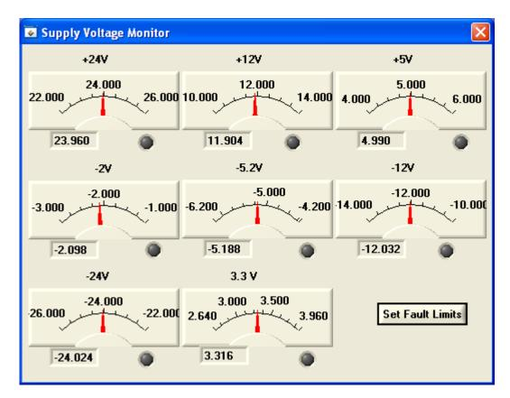
Figure 6-4, Per VXI Rail Voltage Monitoring
