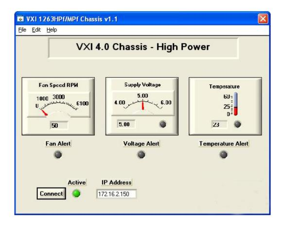
Performance of each cooling fan can be monitored under the "Fan Monitor" sub-menu. An "Alert" light will illuminate if any failure is detected. There are a total of 15 fans in the HPf chassis and their performance can be monitored on four separate sub-menus.
