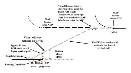
NOTE: Pilots conducting a nonprecision approach must verify lateral alignment with the runway centerline when determining when to descend from MDA. The actual lateral course alignment can vary depending upon the facility type, distance from the facility, or the signal variations which can cause an offset from the intended course centerline.
