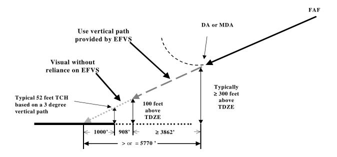
(3) Example Nonprecision Approach Without VNAV. To prevent controlled flight into terrain (CFIT) on nonprecision approaches, the FAA recommends a stabilized constant rate of descent that will safely clear all obstacles along the approach path. When VNAV is not available, another method for achieving a constant rate of descent should be used, such as using a self-computed descent rate or using a FPA reference cue to fly a vertical path that safely clears all obstacles.
